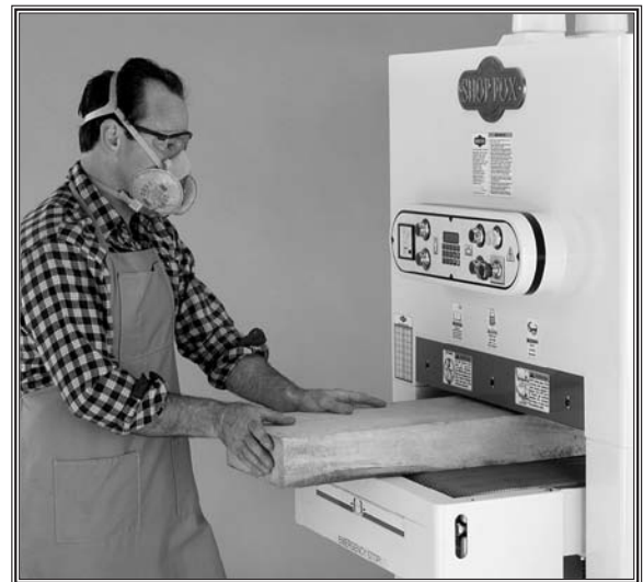
Figure 22. Operator feeding workpiece at correct body position and out of the way of potential kickback.
